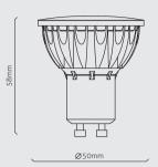
High performance spots with wide beam angle. Perfect solution for lighting where long working hours are required as the aluminium housing provides excellent heat dissipation ability. Available in cold and warm white color temperatures, and in 3 different performance. Recommended for intense household, office or industrial usage.
